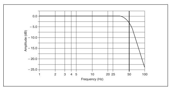
Figure 3. Typical SCC-LP02 Response Curve
